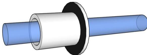
3. Position the outworld portal inside the outworld and push it through one of the holes such that the silicone contacts the inside wall of the outworld.
